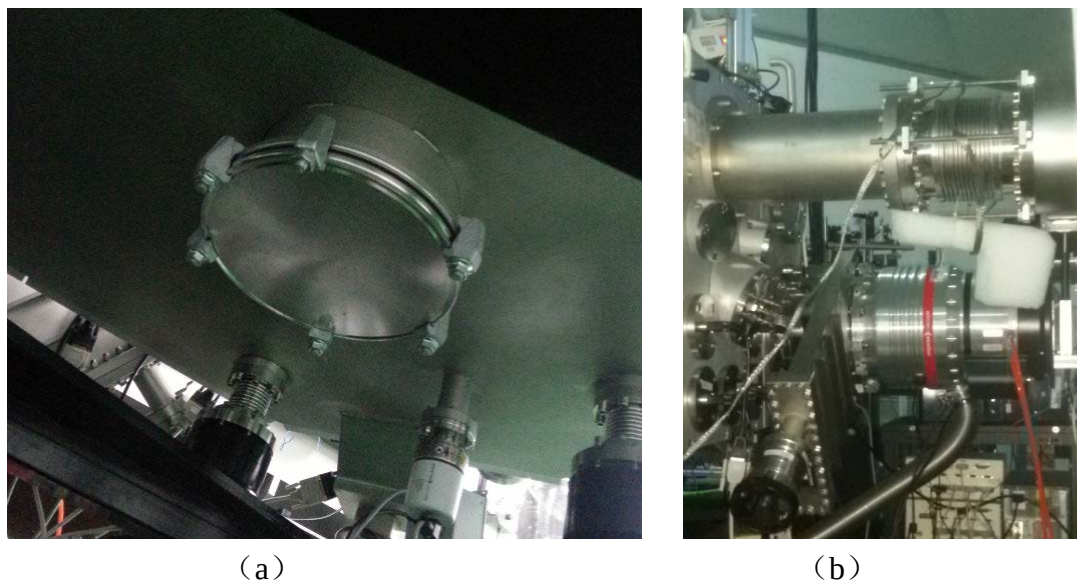
图 2-5 分子泵组位置图 (a) 分子泵位于靶室底部 (当时的接口) (b) 分子泵固定于靶室侧壁 Fig.2-5 The schematic of molecular pump (a) The connection of the molecular pump was under the target chamber (b) Now the pump is installed at the side of the target chamber.
